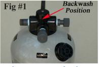
Remove plastic cap from backwash connection, attach garden hose and run to drain.
