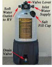
Remove salt fill cap, turn valve lever clockwise back to conditioned water position, open bottom drain valve and drain water from softener, close drain valve.
